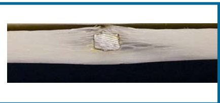
Analysis results have been proven to correlate well to experimental tests – such as this glass/VE composite target subjected to impact
